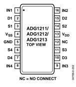
Figure 2. TSSOP Pin Configuration
