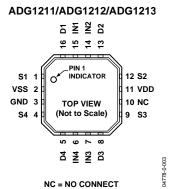
Figure 3. LFCSP Pin Configuration
