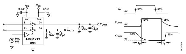
Figure 24. Test Circuit 5—Break Before Make Time Delay
