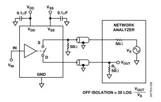
Figure 26. Test Circuit 7—Off Isolation
