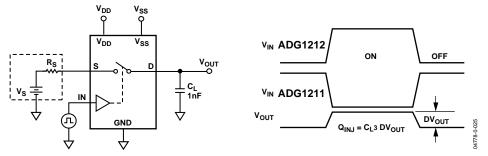
Figure 25. Test Circuit 6—Charge Injection
