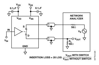
Figure 28. Test Circuit 9—Bandwidth
