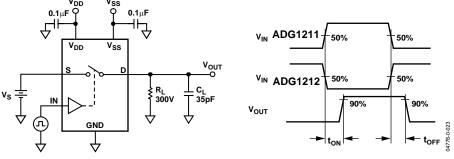
Figure 23. Test Circuit 4—Switching Times
