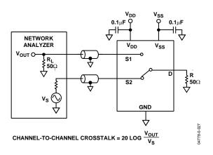
Figure 27. Test Circuit 8—Channel-to-Channel Crosstalk
